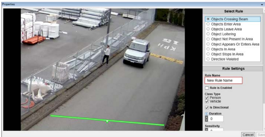
Figure 4: Entering a name for the rule in the Milestone XProtect Management Client.
